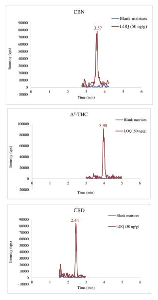
Fig. 1. Chromatograms for blank matrices (dash) and spiked sample at limit of quantification 50 ng/g (solid).
