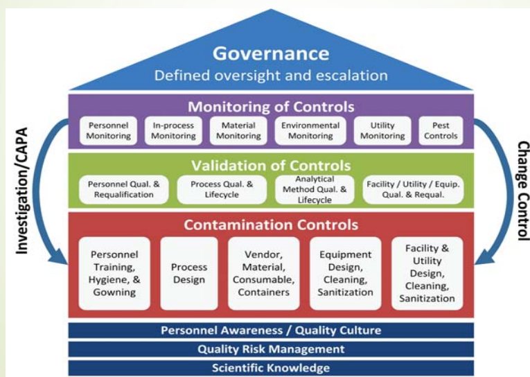
Figure 3.0-1 Elements of a Contamination Control Strategy (courtesy of Sanofi)
