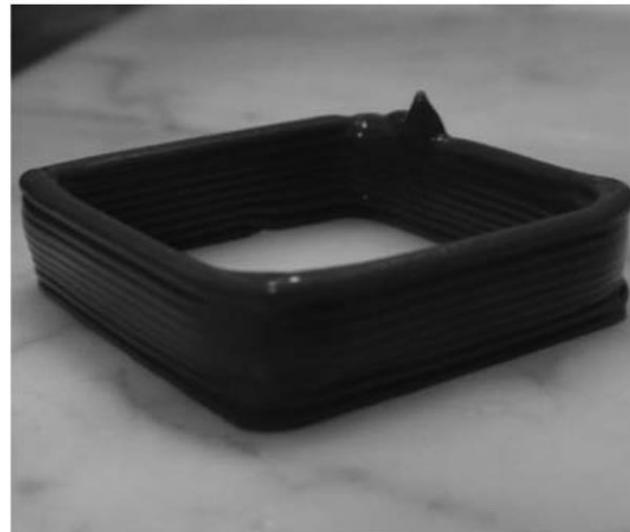
Figure 5. The chocolate square with poor geometrical accuracy.
