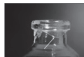
Fold or overlap of glass on the exterior glass surface.
