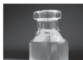
The finish and plane of the seal surface is not perpendicular to the axis of the body.
