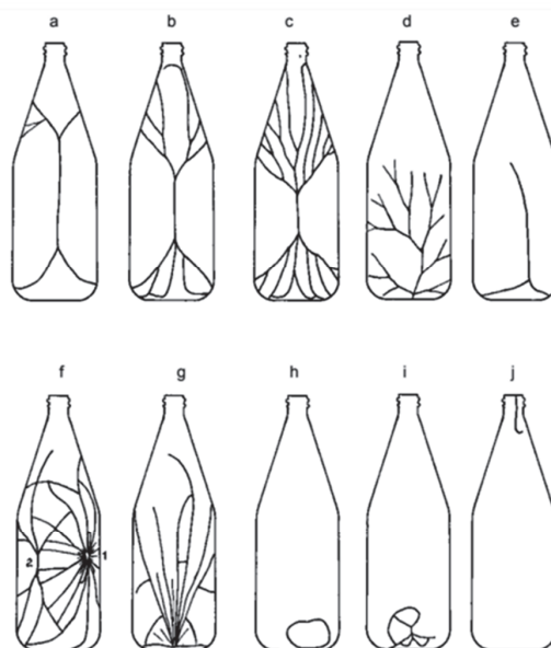
Picture-1: Bottle fracture patterns. (a-c) sidewall fractures due to internal pressure at progressively greater pressures; (d) internal pressure fracture starting from the base; (e) is a thermal fracture from sudden cooling of the base; (f) is an impact fracture on the right side (labeled 1) with a hinge fracture on the side (labeled 2); (g-i) show water hammer fractures and (j) shows a fracture from diametral rim clamping.
