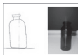
Plane of the container bottom that is not perpendicular to the axis of the body.
