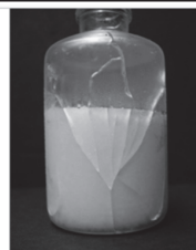
Vial Fracture due to Expansion of Product Component
