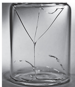
a) Failure at relatively high pressure
