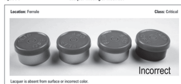
Figure 9-9 Lacquer Missing or Incorrect
