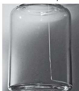
b) Failure at relatively low pressure
