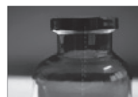
Finish not concentric with the body.
