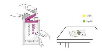
(!) Do not squeeze all the solution out of the extraction tube.
