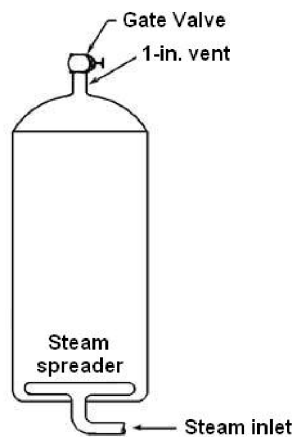
Figure 8: Installation of the vents.
