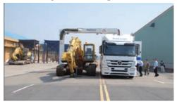
Fig. 7-5 Mobile container x-ray inspection system improves the investigation efficiency
