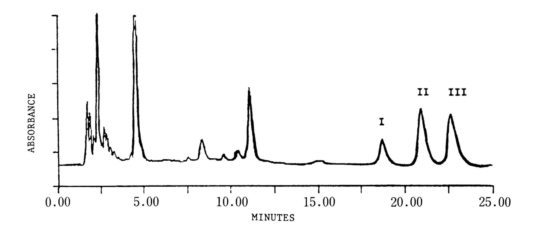
Figure 1. A typical chromatogram of the enantiomeric resolution of S-ibuprofen (II) and R-ibuprofen (III) as their para-nitrobenzylamides in plasma. The internal standard is shown as peak I.
