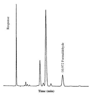
**Figure 2.** HPLC chromatogram of formaldehyde derivated with 2,4-DNPH.
