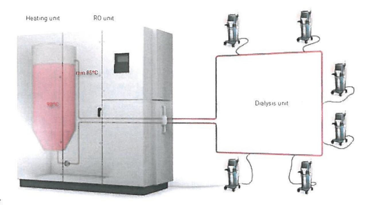
On-line heat disinfection principle
