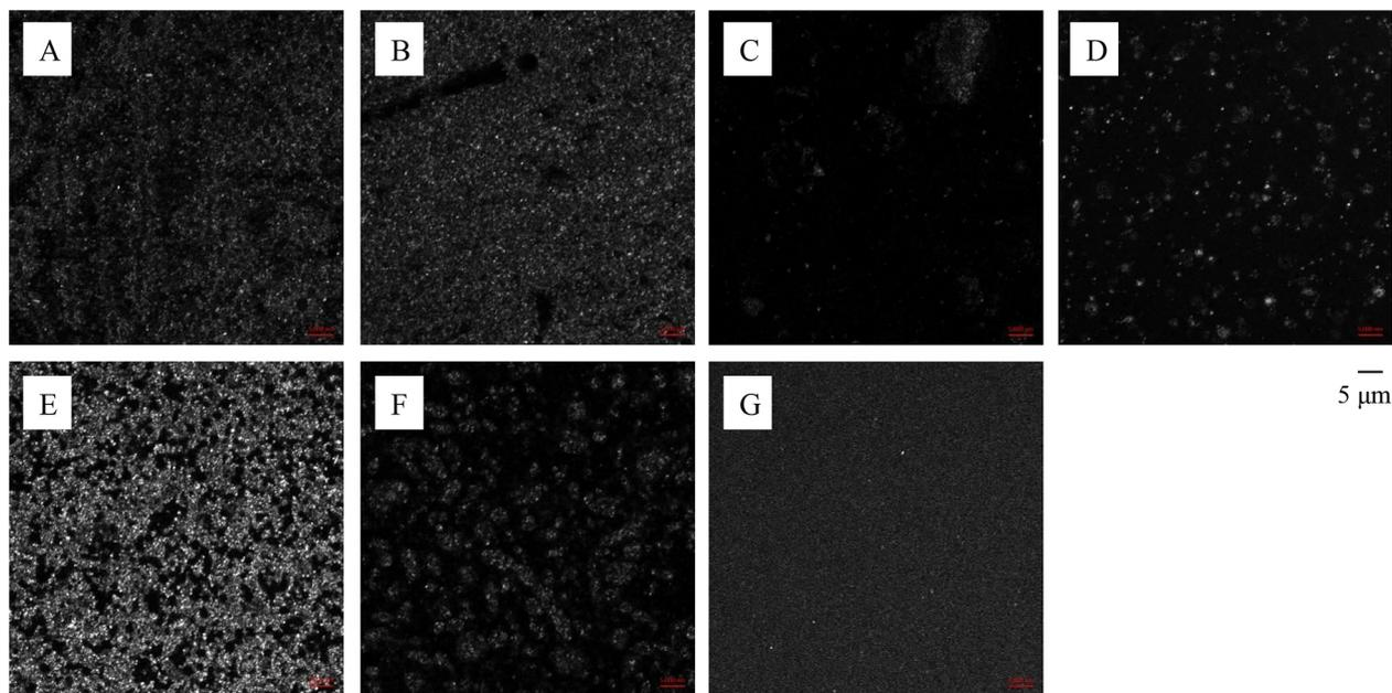
**Fig. 3** – Laser-scanning confocal microscopy of commercial sunscreens containing inorganic nanoparticles in reflectance mode. (A) COM 1, (B) COM 2, (C) COM 3, (D) COM 4, (E) COM 5, (F) COM 6, and (G) ZnO nanoparticle standard. The microscope was equipped with a 561 nm HeNe laser and a 63 × objective (NA1.4). Scale bars represent 5 μm.
