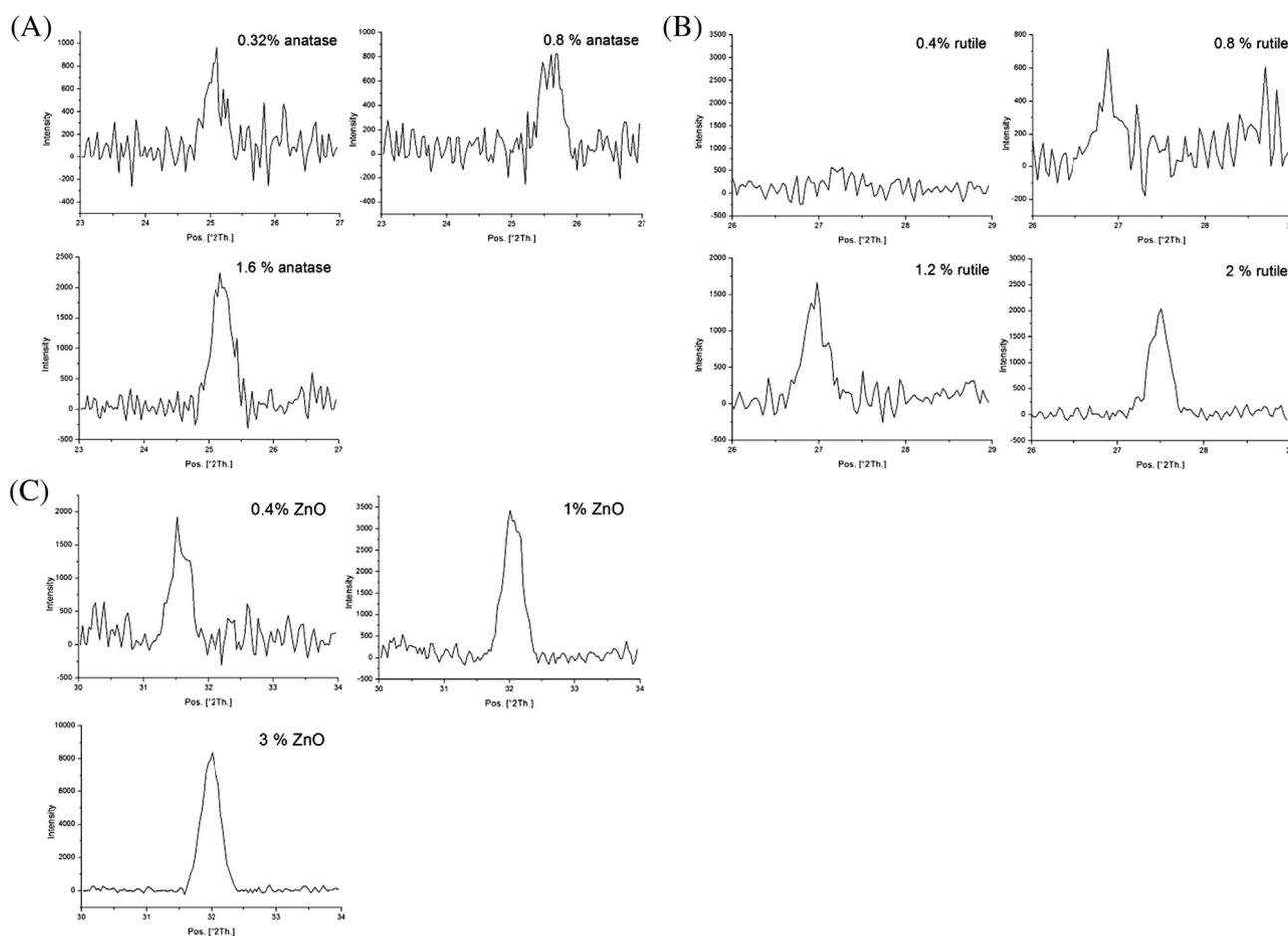
**Fig. 5** – X-ray diffraction patterns of anatase  $\text{TiO}_2$ , rutile  $\text{TiO}_2$ , and ZnO nanoparticle controls at different concentrations. (A) Diffraction patterns of anatase  $\text{TiO}_2$  controls. (B) Diffraction patterns of rutile  $\text{TiO}_2$  controls. (C) Diffraction patterns of ZnO controls.
