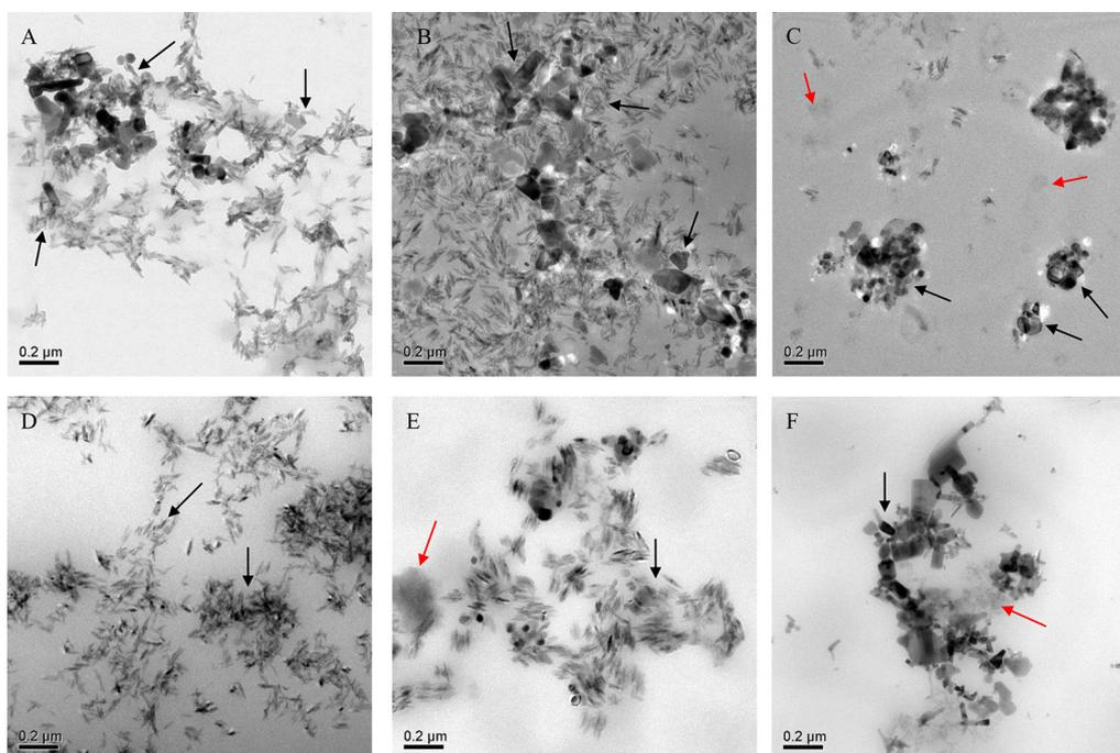
**Fig. 6 – Transmission electron microscopy of commercial sunscreens containing inorganic nanoparticles. (A) COM 1, (B) COM 2, (C) COM 3, (D) COM 4, (E) COM 5, and (F) COM 6. Images were acquired at a beam intensity of 200 kV and a magnification of 10,000–20,000 $\times$ . Black and red arrows indicated metal oxide NPs and the formulation matrix, respectively.**
