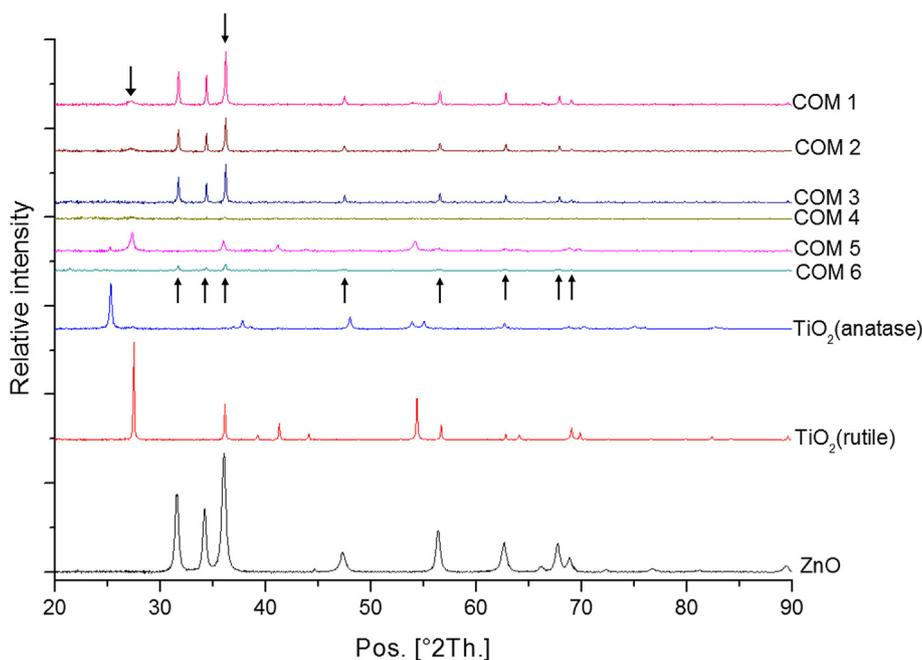
**Fig. 4** – X-ray diffraction patterns of commercial sunscreens COM 1–6 compared with anatase TiO<sub>2</sub>, rutile TiO<sub>2</sub>, and ZnO. Downward arrows indicate the 2θ positions for reflections arising from the rutile phase of TiO<sub>2</sub> and upward arrows indicate 2θ positions for reflections arising from the ZnO wurtzite structure.
