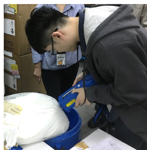
Figure4-4 Demonstration of Raman inspection for the active pharmaceutical ingredients
