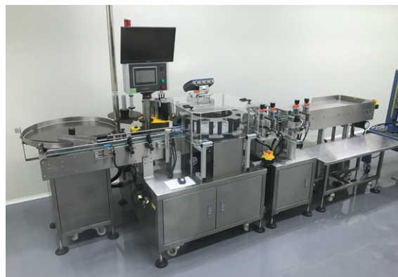
Figure 4-2 Solutions Production Line Equipment-automatic Round Bottle Labeling Machine
