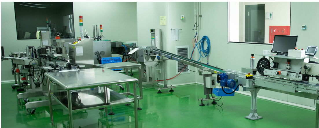
Figure4-2 Ampoule labelling machine , Enload cartoner & Tamper-Evident Labeler
