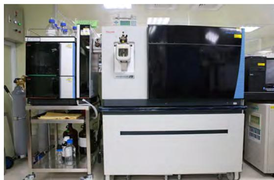
Figure 6-4 Orbitrap Fusion Lumos Tribid Mass Spectrometer (Lumos)
